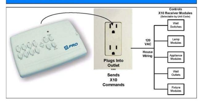
**Description:** The MC10A Mini-Controller gives you manual control of up to eight X10 Receiver Modules of various formats. Just plug it in and you are in control! The MC10A turns On/Off up to eight X10 lights and appliances connected to X10 Receiver Modules. The MC10A has On/Off, Bright/Dim, All Lights On and All Units Off Command Buttons. The Selector Switch assigns the 4 On/Off Buttons to control the X10 Receiver Modules set to Unit Codes 1-4 or 5-8.
