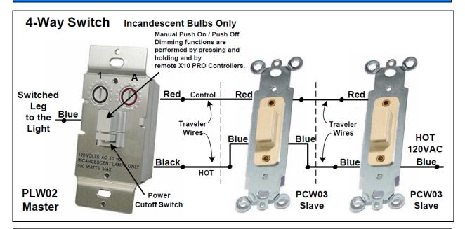
**Description:** The PLW02 3-Way Toggle Style Wall Dimmer Switch Kit is designed to control incandescent bulbs (only) with a rating of 40 to 500W. A pushbutton is provided for local On/Off and Bright/Dim control on the Master and a single push button on the Slave Switches provide the same (see dimming section below). A Power Cutoff Switch located directly below the Local On/Off Pushbutton on the Master Switch is provided for bulb changing. Both switches should line-up for normal operation.
