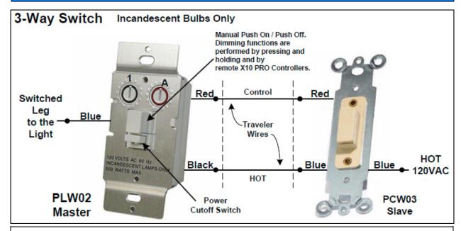
**Description:** The PLW02 3-Way Toggle Style Wall Dimmer Switch Kit is designed to control incandescent bulbs (only) with a rating of 40 to 500W. A pushbutton is provided for local On/Off and Bright/Dim control on the Master and a single push button on the Slave Switch provides the same (see dimming section on back page). A Power Cutoff Switch located directly below the Local On/Off Pushbutton on the Master Switch is provided for bulb changing. Both switches should line-up for normal operation.
