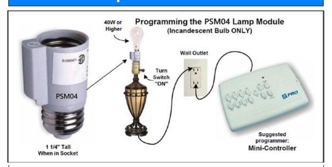
**Description:** Unlike conventional X10 PRO Modules, the PSM04 Screw-in Lamp Module does not have any House and Unit Code Wheels. You setup the Address Codes over the electrical power lines of the home from an X10 PRO Controller (such as a PMC01 Mini-Controller). The Screw-in Lamp Module "remembers" its Codes even after power outages. Because of its ability to remember the Codes (powered off), you can setup the PSM04 at any lamp fixture and then move it to its final destination.
