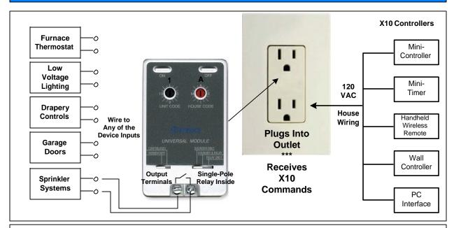
**Description:** The PUM01 Universal Module RECEIVES X10 ON/OFF Signals and it Closes/Opens its internal Single-pole relay switch. The PUM01 is used to operate furnaces via their low-voltage thermostat wires, low voltage lighting, drapery controls, garage door openers, sprinkler systems, etc. The PUM01's internal switch relay is a path interrupter for devices which are not powered above 24VDC (5A) or 30VAC (3.3A).
