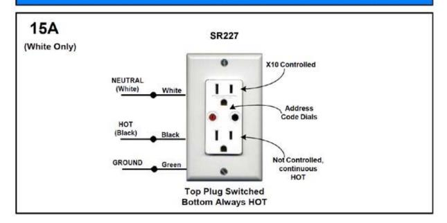
**Description:** The SR227, 15A Duplex Receptacle (NON-DIMMING) is used as a Remote Load Switching Module, which responds to X10 ON/ OFF Commands from an X10 controller. Loads may be plugged into the top receptacle for switching, bottom is always ON. A Trim Plate is included.
