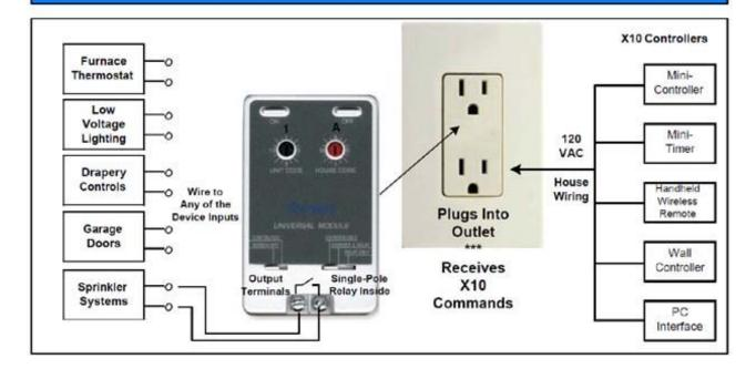
Description: The UM506 Universal Module RECEIVES X10 ON/OFF Signals and it Closes/Opens its internal Single-pole relay switch. The UM506 is used to operate furnaces via their low-voltage thermostat wires, low voltage lighting, drapery controls, garage door openers, sprinkler systems, etc. The UM506's internal switch relay is a path interrupter for devices which are not powered above 24VDC (5A) or 30VAC (3.3A).
