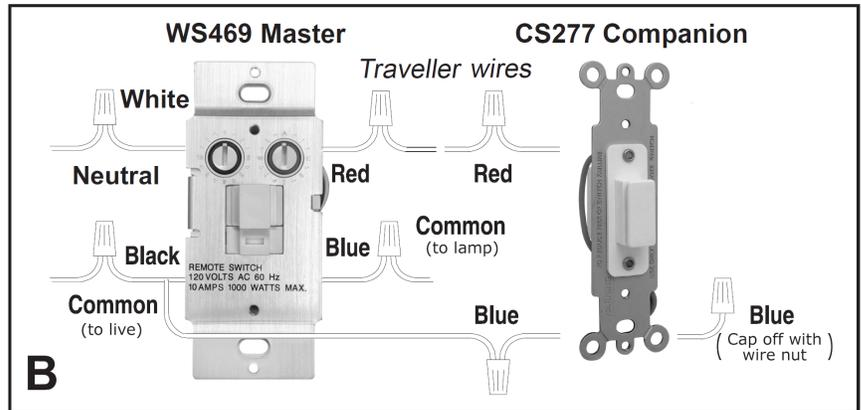
The WS469 is designed to control Lighting and Appliances up to 10Amp 1000 Watts. The switch can replace a single switch, however, it can also be used where two switches control the same light (3-way). In this case a Companion Switch (CS277) is required and is sold separately. A push-button is provided on each switch for local on/off control.
