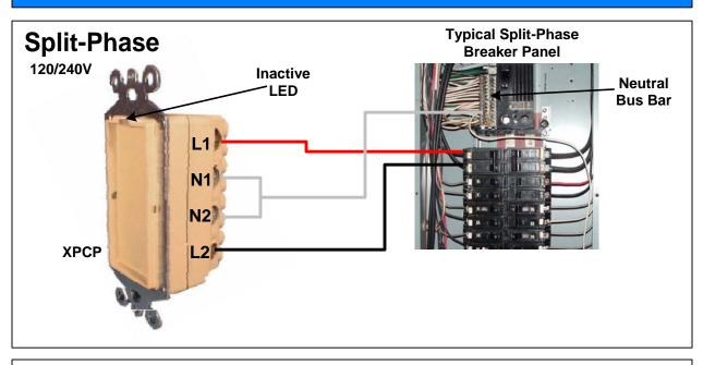
**Description:** The X10 PRO Phase Coupler - Passive serves as a 1:1 signal-bridge across Split-Phase Systems. The XPCP accepts X10 Controller Commands from one phase (L1), and passes (1:1) the X10 Command to the other phase (L2). The XPCP performs this function in both directions, i.e. - (L1 to L2 or L2 to L1). The XPCP's Red LED is inactive. The XPCP is NOT a filter. The above drawing is a simple representation of the XPCP's basic elements of installation. See note below.
