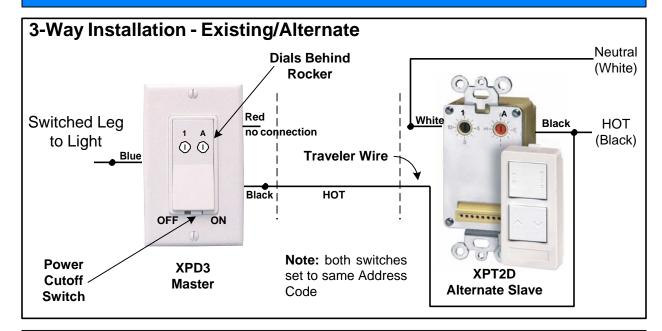
Installation: for 3-Way / 4-Way operation - Existing/Alternate
