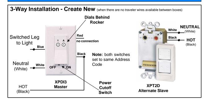
Installation: for 3-Way operation - Create New (when there are no traveler wires available between boxes)
