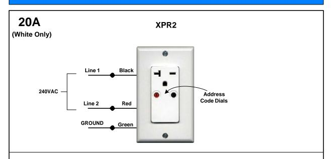
**Description:** The XPR2, 240VAC / 20A Single Receptacle (Non-Dimming) is used as a Remote Load Switching Module, which responds to X10 ON/OFF Commands from an X10 PRO Controller. Great for controlling dust-collectors from a home wood shop and /or small air-conditioning units.
