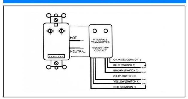
**Description:** The XPT3 Interface Transmitter is a wall mounted controller capable of transmitting from a standard, single gang wall box having HOT and NEUTRAL.
