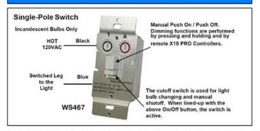
Description: The WS467 Wall Dimmer Switch is designed to control incandescent bulbs (only) with a rating of 40 to 500W. Bulbs rated below 40W may flicker and/or operate erratically. A pushbutton is provided for local On/Off control and manual bright / dimming operation. A Power Cutoff Switch located directly below the Local On/Off Pushbutton is provided for bulb changing. Both switches should line-up for normal operation.
