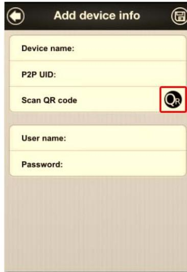
The App auto-opens your smartphone's camera. Place your phone over the QR code on the bottom of the camera, when it comes into focus your phone will take a photo and the App will add the camera's P2P UID automatically.
