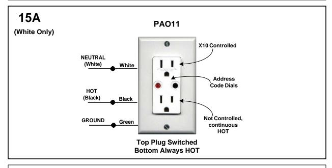
**Description:** The PAO11, 15A Duplex Receptacle (NON-DIMMING) is used as a Remote Load Switching Module, which responds to X10 ON/ OFF Commands from an X10 PRO controller. Loads may be plugged into the top receptacle for switching, bottom is always ON. A Trim Plate is included.
